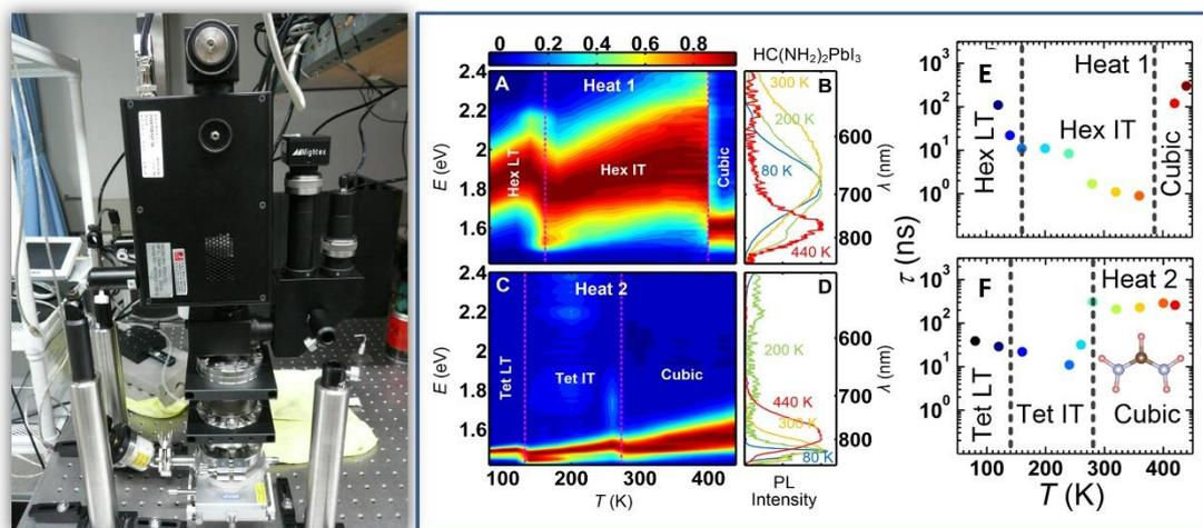
Figure 1 : (left) The Variable Temperature Laser Scanning Conjugate Focus Spectroscopy Microscope built by the Taiwan team. (right) Upon two different heating processes, the temperature-dependent photoluminescence spectra (A, D) and time-resolved photoluminescence lifetime (E, F), when  $\text{FAPbI}_3$  goes into a cubic phase, significant increases of photoluminescence lifetime are observed upon both processes.
