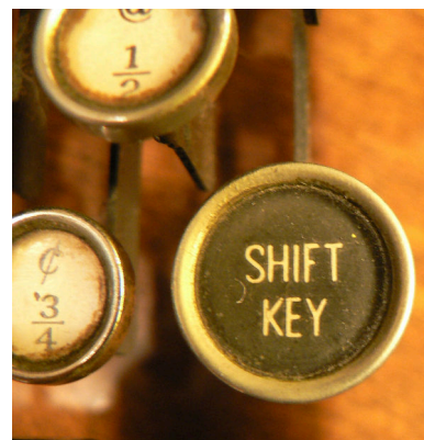
Figure 13.11: If you’ve never used a typewriter, you might not know that the shift key originally shifted part of the typewriter up or down, to get access to upper-case letters. This reduced the number of keys that were needed. Before the shift key was invented typewriters either had separate keys for each upper and lower case letter, or they could only type in upper (or lower) case.
