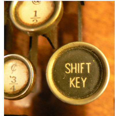
Figure 13.11: If you’ve never used a typewriter, you might not know that the shift key originally shifted part of the typewriter up or down, to get access to upper-case letters. This reduced the number of keys that were needed. Before the shift key was invented typewriters either had separate keys for each upper and lower case letter, or they could only type in upper (or lower) case.
