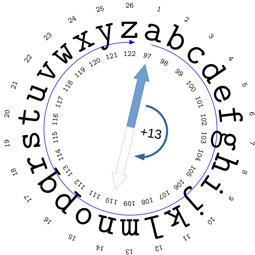
Figure 13.10: Adding 13 to the value 'a' moves halfway around the circle to 'n'. Adding 13 again would bring us back to 'a'.
