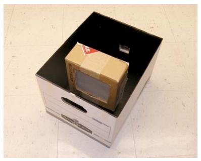
9.) This picture of the experimental set-up showing our closed pinhole box pointed at the object we will view (a 100-Watt white frosted light bulb). All viewing should be done in a dark room. University of Virginia Physics Department PHYS 6251, PHYS 6252, PHYS 6253
