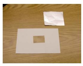
2.) Tape the foil over the opening in the index card with masking tape (or some similar kind of tape).
