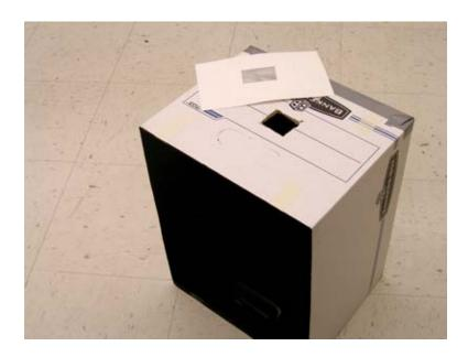
6.) To make the image viewing screen - take your smaller box, cut a large square in one end, and tape a piece of wax paper over the opening.
