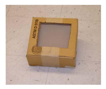
8.) Insert the small box (target screen) inside the big box (as shown). This picture illustrates the relationship between the pinhole foil (in the front of the box), the target screen (inside the box), and the back viewing opening in the back. Put the top on the big box and you are ready to go.
