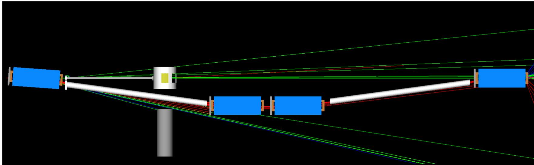
While these both moved the dump away from the pivot they suffered from the 'sheet of flame' - the dispersion of the beam after the dipole due to bremsstrahlung and multiple scattering in the radiator
