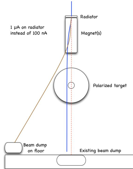
Separated function dipole and dump
