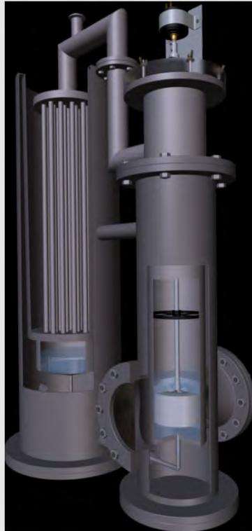
Argon cooled cryostat
