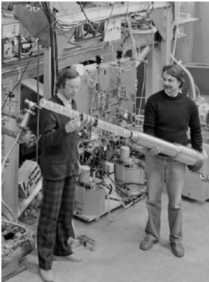
1 m long target for muon beams (T. Niinikoski on the left)
