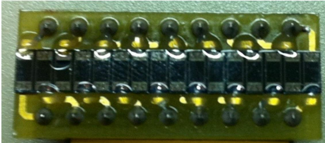
Linear Photodiode Array
